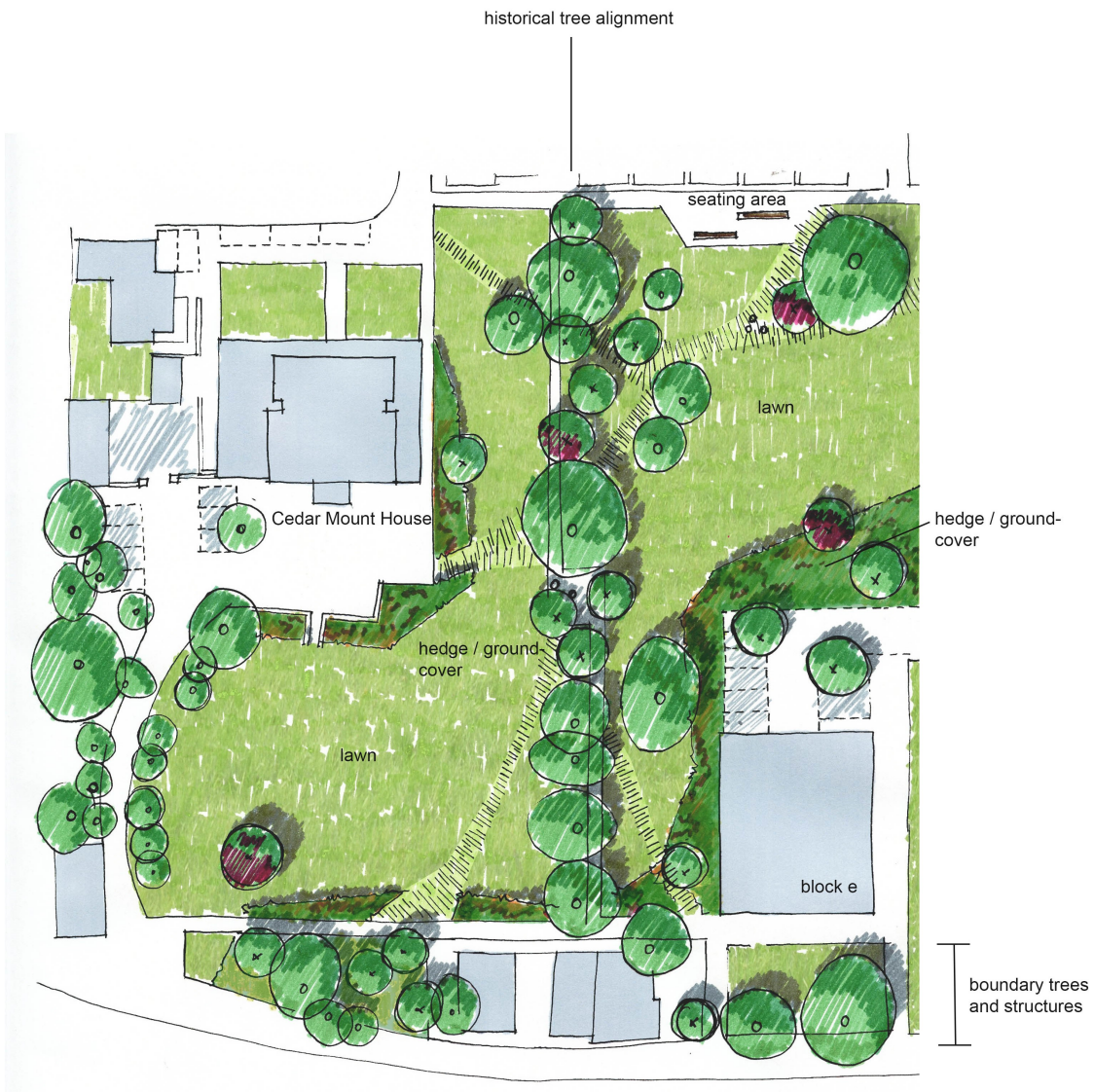
Figure 8: Design development sketch showing the main design considerations of the landscape strategy around Cedar Mount House.
